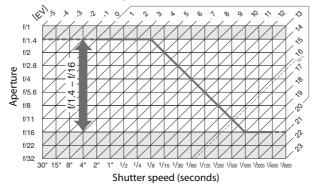
The maximum and minimum values for EV vary with ISO sensitivity; the above graph assumes an ISO sensitivity of ISO 100 equivalent. When matrix metering is used, values over 161/3 EV are reduced to 161/3 EV.
