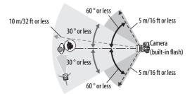
Wireless remote sensors on flash units should face camera.
