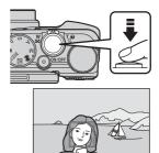
**5** Without lifting your finger, press the shutter-release button the rest of the way down.
