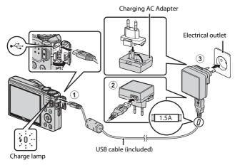
If a plug adapter\* is included with your camera, securely connect it to the Charging AC Adapter. Once the two are connected, attempting to forcibly remove the plug adapter could damage the product.
