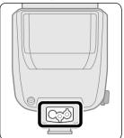
To use an external power source, remove the external power source terminal cover and connect the power cord to the terminal.
