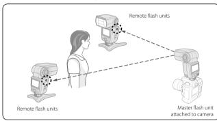
As a basic guide, the effective distance between the master flash unit
