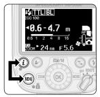
Press the **MENU** button and the *i*. button simultaneously for 2 seconds to reset all settings except menu settings to default
