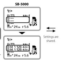
Flash function settings for remote flash units are changed on the SB-5000.
