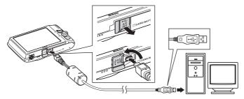
The camera is automatically turned on and the power-on lamp will light. The camera monitor will remain off.
