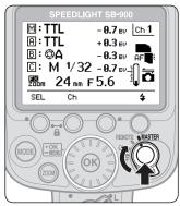
Align the index on the Power ON-OFF switch/wireless setting switch to MASTER.
