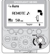
• Align the index on the Wireless setting switch with [REMOTE].
