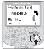
Align the index on the Power ON-OFF switch/wireless setting switch to REMOTE
