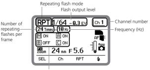
Flash firing of master flash unit and remote flash units (ON/OFF) in Group A (B, C) activated/canceled
