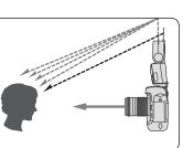
Pull out the bounce card and the wide-flash adapter and, while holding the bounce card, slide the wide-flash adapter back into place inside the flash head.
