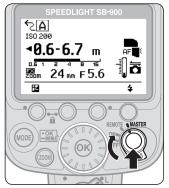
• Align the index on the Wireless setting switch with [MASTER].
