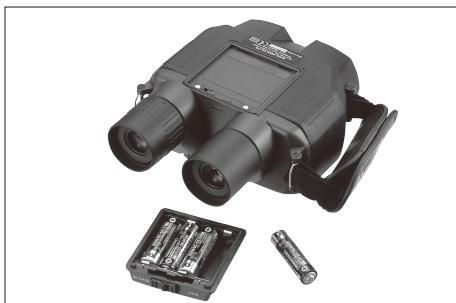
Remove the battery holder and insert the batteries. When returning the battery holder to the binoculars, be certain to seat it properly, with the O-ring in place, and move the slide to the locked position. This seals the binoculars to help keep them waterproof.
