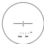
Example of measurement failure
