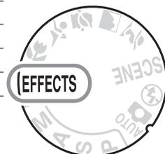
The following effects can be selected by rotating the mode dial to **EFFECTS** and rotating the command dial until the desired option appears in the monitor.
