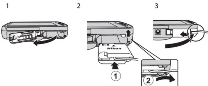
Make sure that the power connector cord has been properly aligned in power connector and battery-chamber grooves before closing the battery-chamber cover. If part of the cord runs out of the grooves, the cover or cord may be damaged when the cover is closed.
