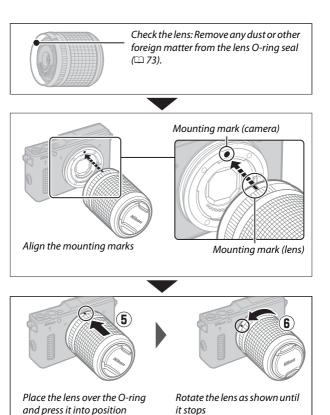
When placing the lens over the O-ring, be careful not to damage the camera or lens; do not use excessive force.
