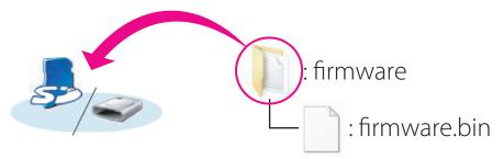
When copying is complete, open the "firmware" folder on the memory card and confirm that it contains the file "firmware.bin".
