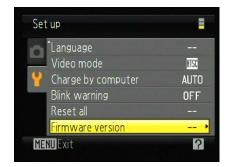
The current firmware version will be displayed. Confirm that the firmware version is the correct version for this update.
