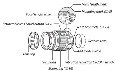
The AF-S DX NIKKOR 18-55mm f/3.5-5.6G VR II features a retractable lens barrel.
