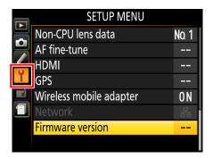
5 The current firmware version will be displayed. Confirm that the firmware version is the correct version for this update.
