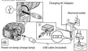
If a plug adapter\* is included with your camera, securely connect it to the Charging AC Adapter. Once the two are connected, attempting to forcibly remove the plug adapter could damage the product.
