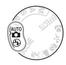
Before proceeding, turn the camera on and rotate the mode dial to or (f) (the only difference between the two is that the flash will not fire in (f) mode).
