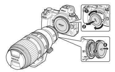
2. Position the lens on the camera body, keeping the mounting mark on the lens aligned with the mounting mark on the camera body (1), and then rotate the lens counterclockwise (2) until it clicks into place.
