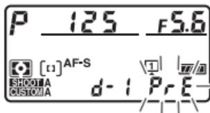
The focus point will change to a white balance target positioned in the center of the frame as shown and cannot be moved. After adjusting lighting to your satisfaction, aim the camera to place the white balance target over the reference object and press the shutter-release button all the way down to measure white balance. You can then press the **WB** button to exit direct measurement mode.
