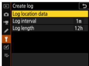
The camera will log its position at the selected interval for the selected time; the time remaining can be viewed by selecting [Location data (built-in)]. To end, pause, or resume recording, highlight [Log location data] and press **OK**.
