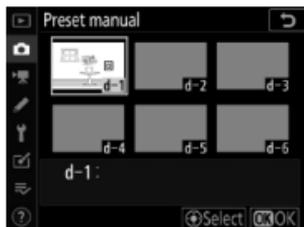
Next, highlight **[Select image]** to view the pictures on the memory card. Highlight the source picture and press **OK** to copy white balance from the source picture to the selected preset.
