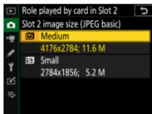
The size of the copies recorded to the card in Slot 2 is shown on the left side of the rear control panel.
