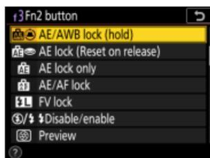
Auto white balance (AWB) lock applies only in [Auto] and [Natural light auto] modes, and both exposure and AWB lock end when the selected control is pressed a second time or the standby timer expires.
