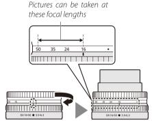
To retract the lens, rotate the zoom ring in the opposite direction, stopping when you reach the  $(\bullet)$  position on the focal length scale.
