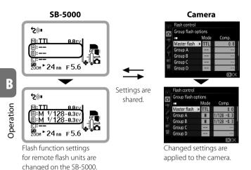
If flash function settings are made on the SB-5000 when not attached to a camera, the configured settings will be applied to the camera after the SB-5000 is attached.
