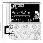
Press the **MENU** button and the ibutton simultaneously for 2 seconds to reset all settings except menu settings to default
