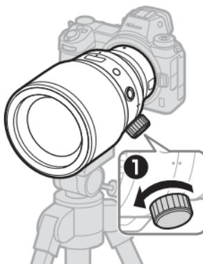
2 Rotate the camera (2) to align the lens rotation index with the tripod collar rotation index that matches the desired orientation (landscape or portrait).
