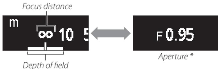
\* Aperture is displayed only when the camera is in mode **A** or **M**. The display for other modes is shown in the illustration.
