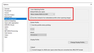
2. Remove the check from [Convert images to sRGB color space when they are converted into JPEG/TIFF format] under [Output] in the [Color Management] panel.
