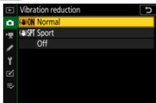
Note that if an F mount lens with a vibration reduction switch is attached via an optional FTZ mount adapter, the **[Vibration reduction]** item in the camera menus will be grayed out and unavailable, and vibration reduction options will instead have to be selected using the switch.
