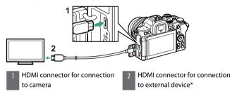
Choose a cable with a connector that matches the connector on the HDMI device
