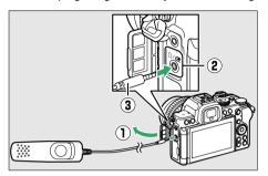
Connect the MC-DC3 remote cord to the headphone/remote cord connector. The MC-DC3 will not function if it is connected to the similar looking external microphone input connector.
