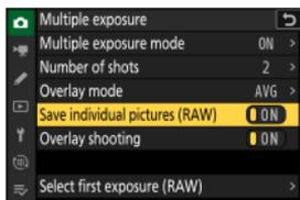
To save both the multiple exposure and the shots that make it up, select [**ON**]; the individual shots are saved in NEF (RAW) format. To save only the multiple exposure, select [**OFF**].
