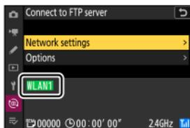
When a connection is established, the profile name will be displayed in green in the camera **[Connect to FTP server]** menu.
