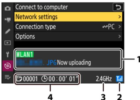
**1 Status:** The status of the connection to the host. The profile name is displayed in green when a connection is established. While files are being transferred, the status display shows “Now uploading” preceded by the name of the file being sent. Errors are also displayed here.
