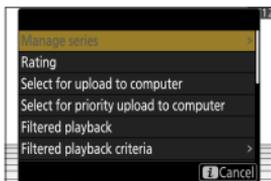
The **i** menu items used to select pictures for upload vary with the type of device connected.
