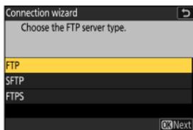
Highlight **[FTP]**, **[SFTP]** (SSH FTP), or **[FTPS]** (FTP-SSL) and press **OK** to display a dialog where you can enter the server address.
