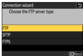
Highlight **[FTP]**, **[SFTP]** (SSH FTP), or **[FTPS]** (FTP-SSL) and press **⏎** to display a dialog where you can enter the FTP server port number.
