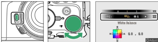
Options for the selected setting, if any, can be chosen by holding the **Fn1** button and rotating the sub-command dial.
