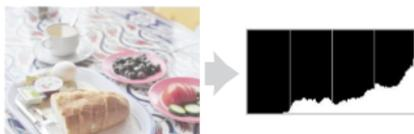
Increasing exposure compensation shifts the distribution of tones to the right, while decreasing exposure compensation shifts the distribution to the
