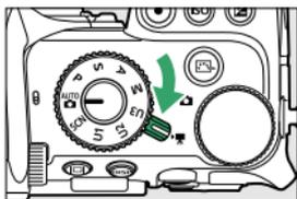
Note that the built-in flash and optional flash units cannot be used when the camera is in video mode.
