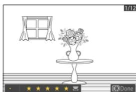
Rotate the main command dial to highlight the desired rating and press **OK** to select. Choose from ratings of from zero to five stars, or select **OK** to mark the picture as a candidate for later deletion.
