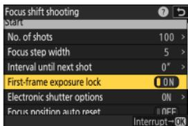
Highlight [**First-frame exposure lock**] and press to select [ON] or [OFF].
