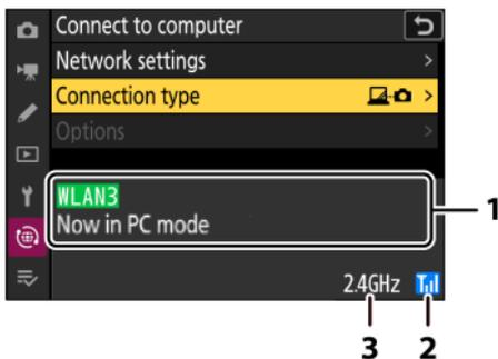
**1 Status:** The status of the connection to the host. The profile name is displayed in green when a connection is established. Errors are also displayed here (□416).
