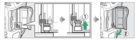
Be careful not to slide the memory card slot cover release latch back down after removing the memory card slot cover. The cover cannot be re-attached with the latch lowered.
