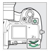
• ☑ icons and exposure indicators appear in the shooting display and control panel. In modes other than M, the zero ("0") at the center of the exposure indicator flashes. The current value for exposure compensation can be confirmed by pressing the ☑ button.
