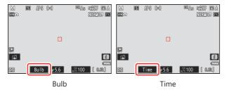
Note that the exposure indicators are not displayed at a shutter speed of **Bulb** or **Time**.
