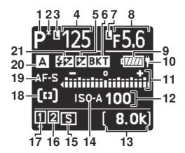
1 Shooting mode (\(\to\) 128) **9** Battery indicator (QQ 86) **2** Flexible program indicator (\(\to \frac{129}{2}\) **10** USB power delivery ( $\bigcirc$  770) 3 Shutter speed lock icon (<u>4661</u>) **11** Exposure indicator **4** Shutter speed (☐ 129, ☐ 130) Exposure ( 131) Exposure compensation value ( 138) • Exposure compensation ( 138) Flash compensation value (412) Exposure and flash bracketing (
