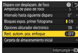
Marque [**Rest. autom. pos. enfoque**] y pulse
