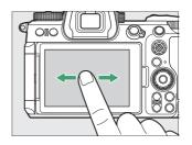
• In full-frame playback, touching the bottom of the display brings up a frame-advance bar. Slide your finger left or right over the bar to scroll rapidly to other pictures.
